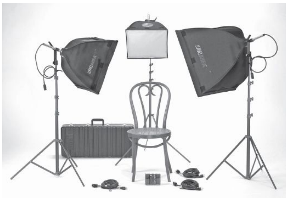
Fig. 12-19. Collapsible soft boxes produce very soft, very even illumination and fold up for travel. Shown here, Lowel Rifa lights of various sizes. See also Fig. 12-13 . (Lowel Light Mfg., Inc.)
