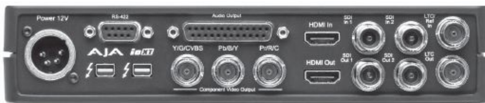
Fig. 14-5. The back of the AJA Io XT shows various connectors. (lower row, left to right): XLR for power; two Thunderbolt ports (one connects to the Mac, the other can daisy-chain to storage or other peripherals); BNC jacks for SD or HD component video out (composite video is on the Y connector); HDMI out (carries video, audio, and timecode); 3G/HD/SD-SDI out; and LTC (timecode) out. (AJA Video Systems)
