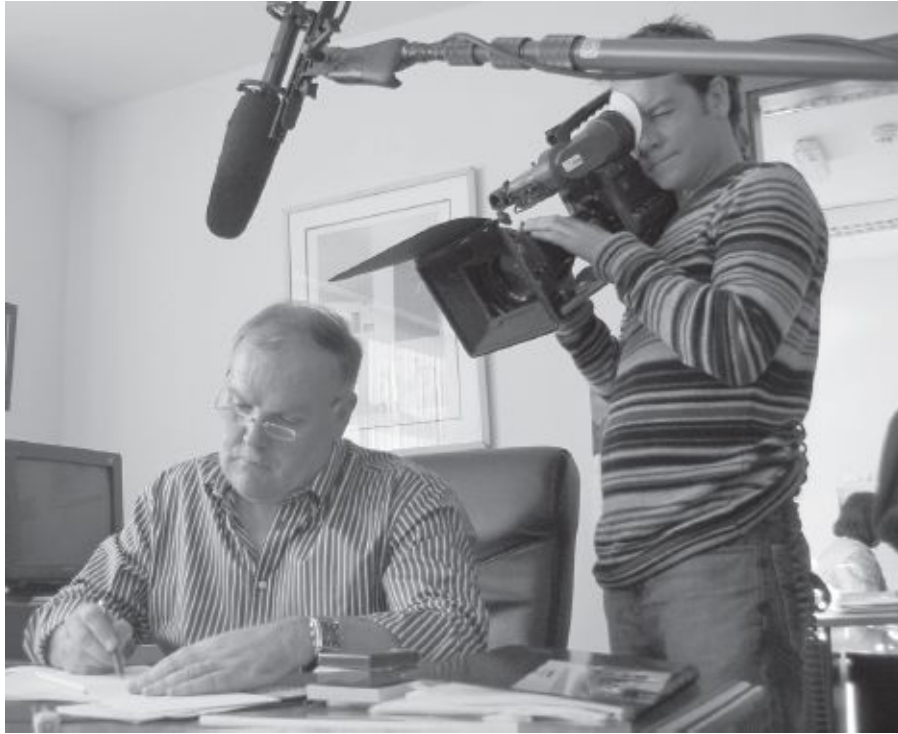
Fig. 8-10. The French flag attached to the top of the matte box (also called an eyebrow) helps block light sources from above. (Bob Corkey)
