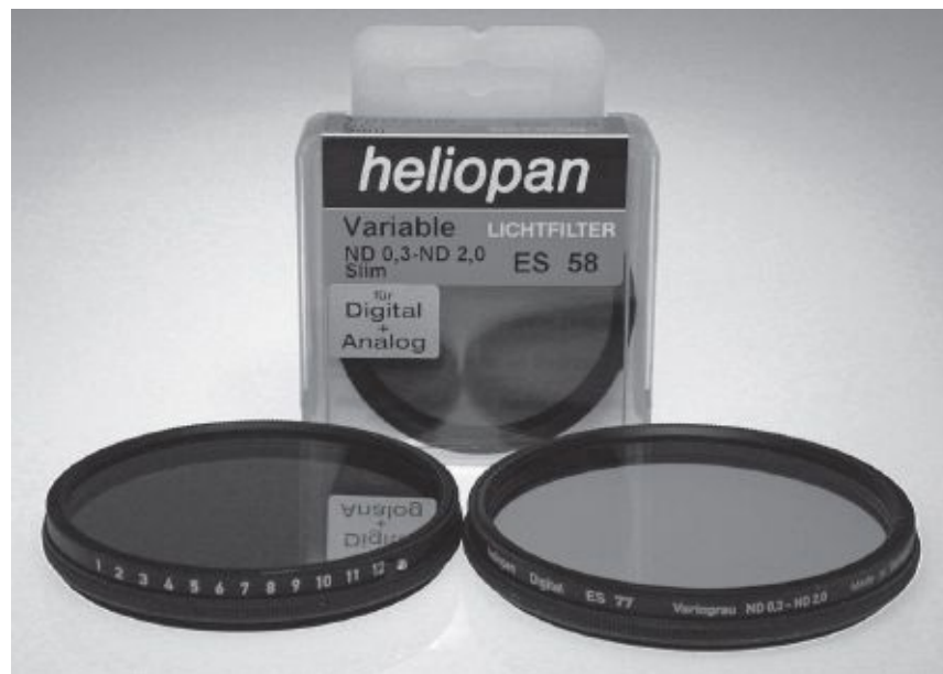
Fig. 8-6. Variable neutral density filters. Also called faders, variable NDs allow you to dial in different amounts with one filter. The Heliopan model shown ranges from 0.3 ND (one stop) to 2.0 ND (six and two-thirds stops). (HP Marketing Corp.)
