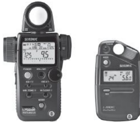
Fig. 7-12. Sekonic digital meters that can take both incident and reflected readings. (left) L-758DR. (right) L-308DC. (Sekonic)
