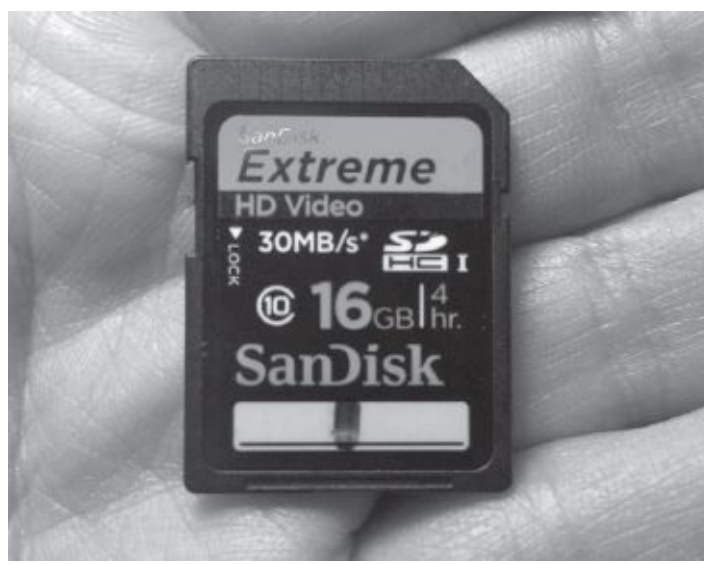
Fig. 1-26. Secure Digital High Capacity (SDHC) flash memory card. When buying cards, be sure the read/write speed is sufficient for the video format you're recording. This card is rated at 30 MB per second. (Steven Ascher)
