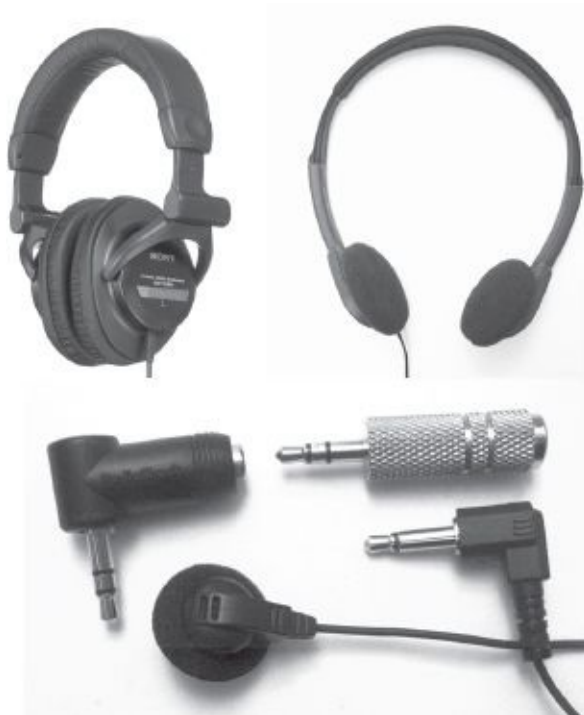
Fig. 11-2. (upper left) Headphones with closed ear pads. (upper right) Headphones with open ear pads. (bottom) Mono earpiece shown with mono connector; stereo-to-mono adapter (so you can hear both channels from the camcorder); and right-angle adapter (so the plug doesn't stick out from the camcorder).
