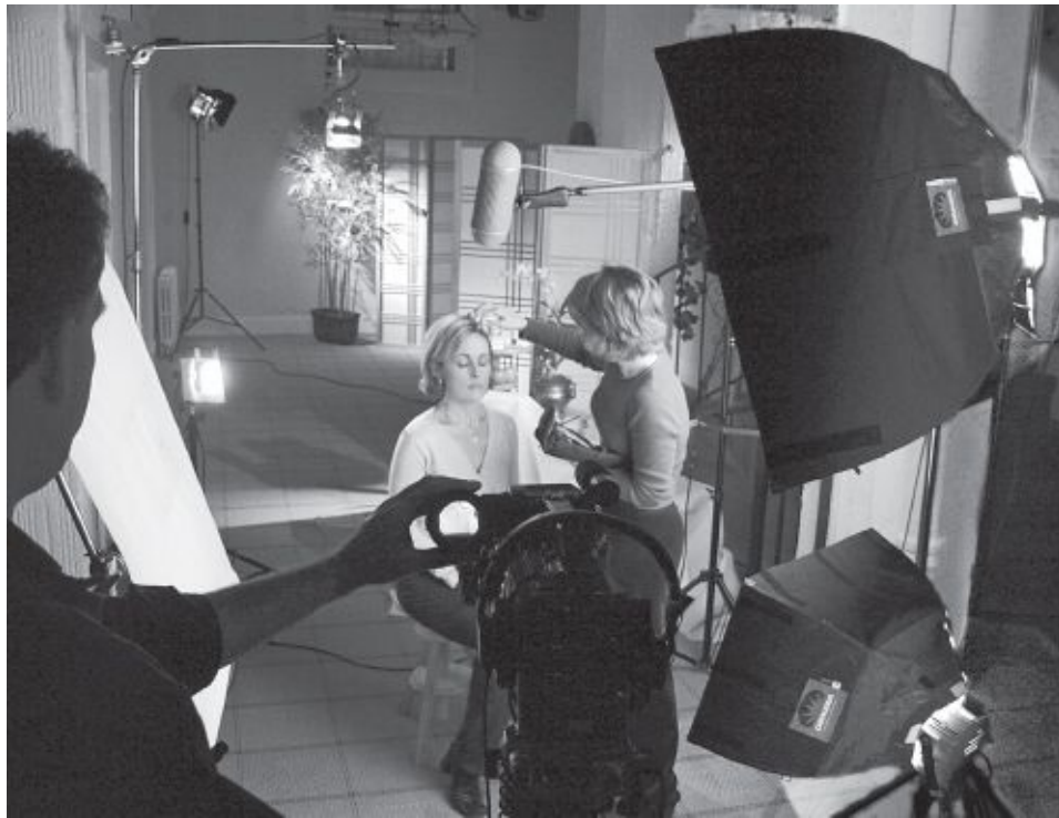
Fig. 12-20. Chimera lightbanks being used for soft key lighting. A reflector provides fill. See the results in Fig. 12-29D . (Chimera)
