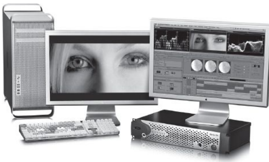
Fig. 5-22. When editing video, it's important that tonal values be correctly translated from the editing system any built-in or external monitors. Shown here, Avid Nitris DX input/output and monitoring interface. (Avid Technology, Inc.)
