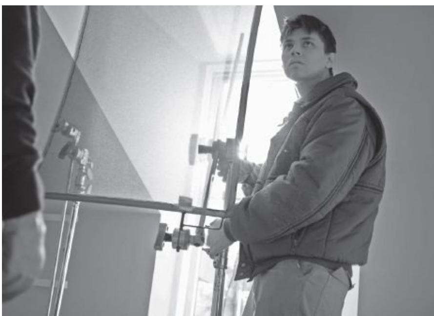
Fig. 12-25. Adjusting a double scrim on a grip stand. Useful for shading off the light on part of a scene.
