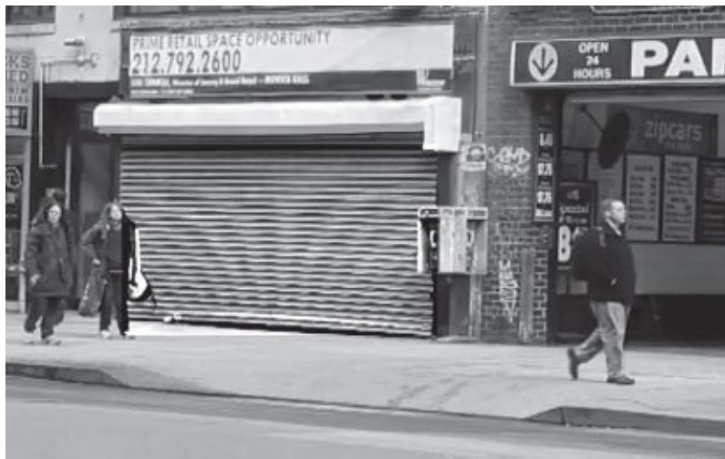
Fig. 5-18. Moiré. The metal gate on the storefront has only horizontal slats, but this video image shot with a DSLR (Canon EOS 5D Mark II with full-frame sensor) shows a fan pattern of moving dark lines. This is one of several types of moiré that can occur in video, particularly with footage from DSLRs. (David Leitner)
