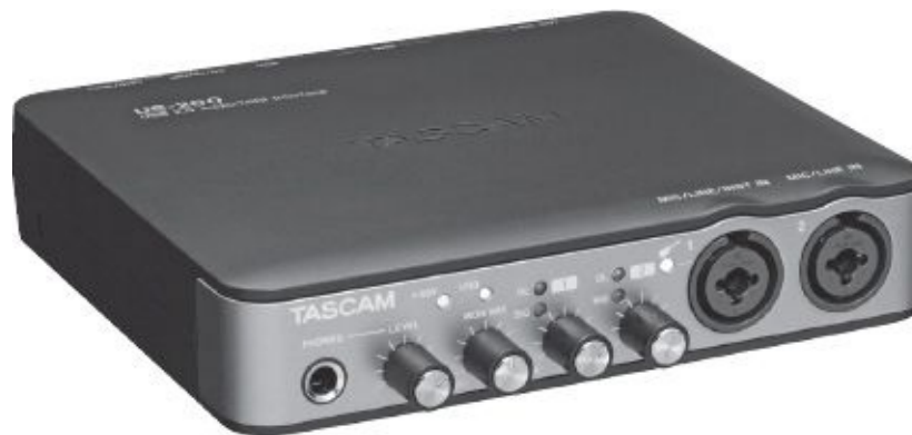
Fig. 10-8. A mic preamp like the Tascam US-200 allows you to input mics that have professional XLR connectors to a computer. Digitizes audio at up to 96 kHz/24-bit resolution. Can supply phantom power to mics that require it. (TASCAM)
