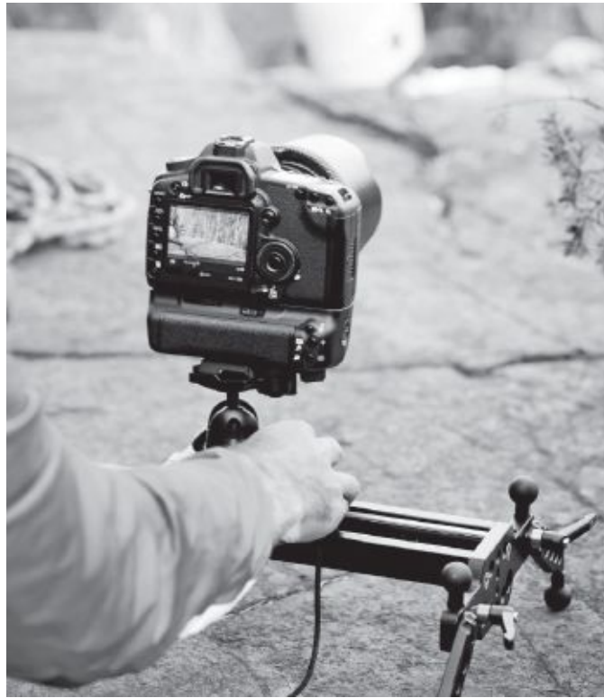
Fig. 1-19. DSLRs provide affordable, compact HD recording, usually with some compromises in audio quality and sometimes artifacts in the recorded picture. Shown here with slider for side-to-side movements. (Cinevate)
