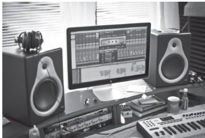
Fig. 15-2. Digital audio workstation (DAW). Most DAWs, including the Pro Tools system shown here, can be used for movie track work and mixing, as well as creating music. (Avid Technology, Inc.)
