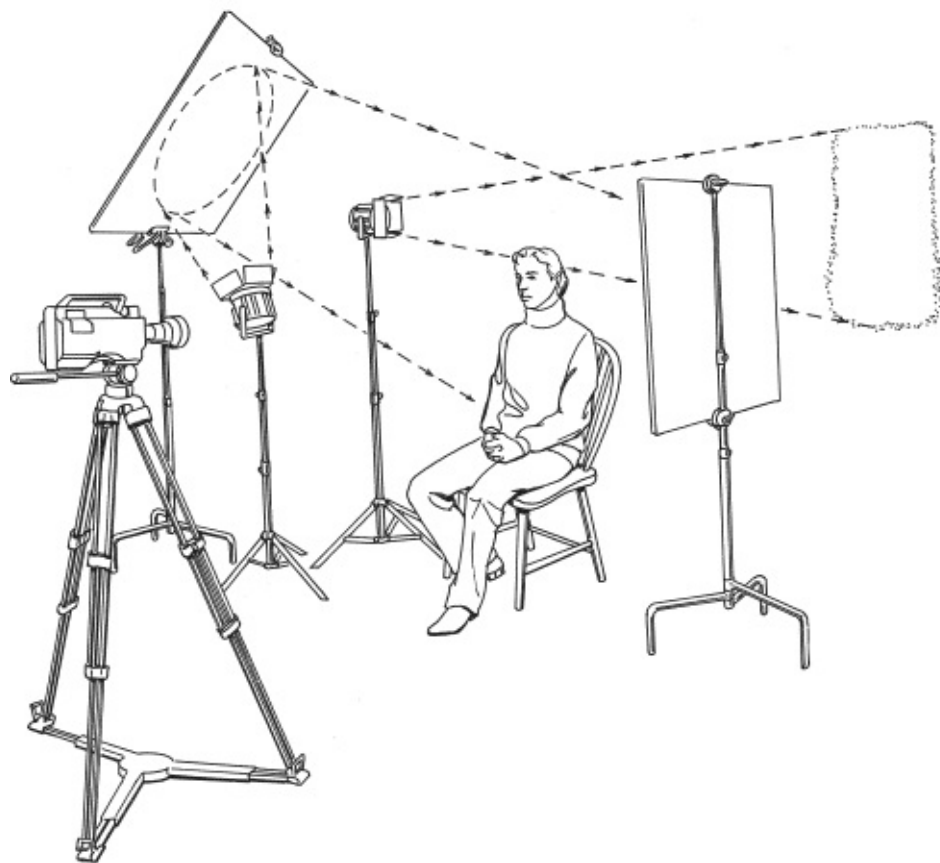
Fig. 12-34. “Window-lit” scene. A lighting setup that might be used to simulate the light in Fig. 12-33 . Key light is bounced for a soft look. Fill lighting is provided by a white card just out of frame to the right. A set light provides the sun effect on the back wall. Flags and/or a cookie might be needed to create the desired effects on the walls. Compare with Fig. 12-37 . (Robert Brun)
