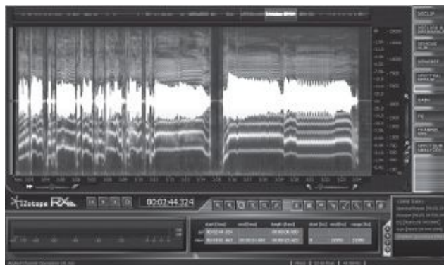
Fig. 15-18. Digital noise reducers, like the iZotope RX 2, can target many types of noise and reduce or remove them, often with little effect on dialogue and music. The RX 2 is available as a plug-in and a stand-alone application. Most NLEs offer some form of noise reduction. (iZotope, Inc.)
