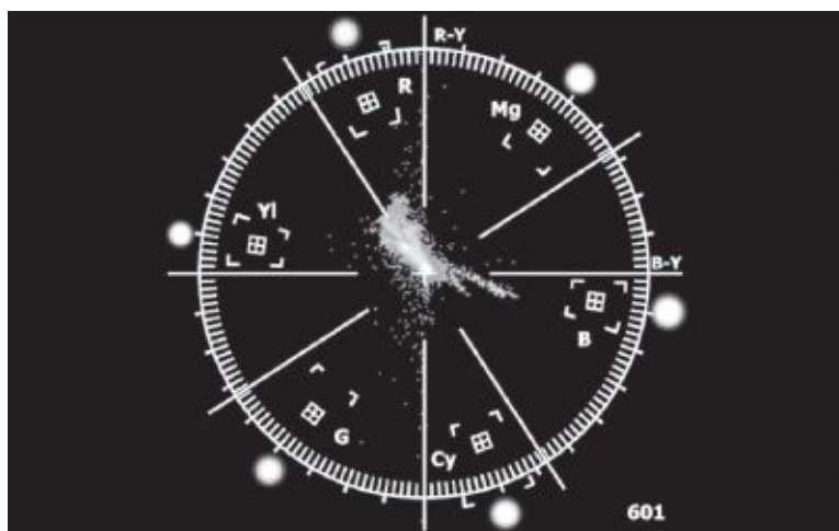
Fig. 8-3. The vectorscope shows color information. This scope, part of Adobe Premiere Pro, is displaying standard definition (Rec. 601) video. (Adobe Systems, Inc.)
