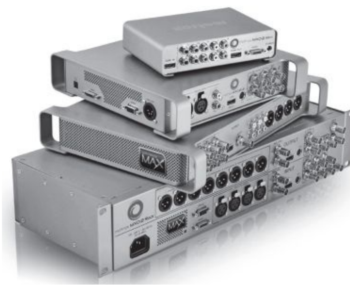
Fig. 5-23. Matrox’s MXO2 family offers a range of input/output (I/O) and monitoring options to use with editing apps like Adobe Premiere Pro, Apple Final Cut Pro, and Avid Media Composer. Various models offer I/O via HDMI (RGB or Y' C_B C_R ), HD-SDI, SDI, and other connectors. The HDMI calibration utility lets an RGB monitor perform like a broadcast HD video monitor with proper display of Rec. 709 component color space so it can be used for color grading. (Matrox Electronic Systems, Ltd.)
