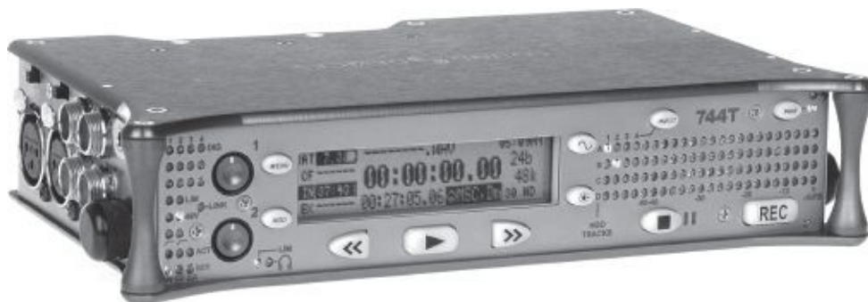
Fig. 10-4. The Sound Devices 744T is a file-based digital recorder that can record up to four audio tracks to an internal hard drive, CompactFlash cards, or external FireWire drives. This and similar
