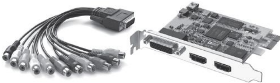
Fig. 14-6. Blackmagic Design's Intensity Pro is an affordable input/output card that allows you to connect an HDMI video monitor to a desktop computer via its PCI Express slot. Can also be used to capture HDMI directly from a camera, bypassing the camera's internal compression. Breakout cable on left provides connections to analog video and audio gear. The Intensity Extreme can be used with a laptop. (Blackmagic Design)
