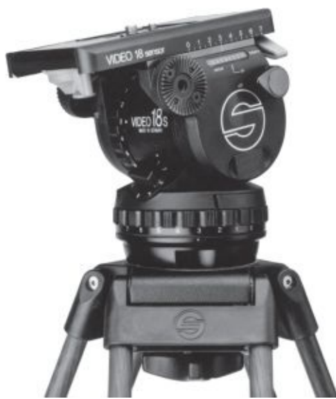
Fig. 9-37. Fluid heads are the most versatile and easiest to operate. This Sachtler head has seven-step pan and tilt drag controls and a quick-release plate that attaches to the camera and can be snapped on and off the head. The top surface slides forward and back for balance. (Fletcher Chicago/Sachtler Corp. of America)
