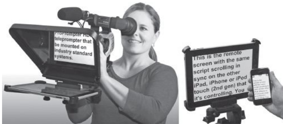
Fig. 9-33. Teleprompter. (left) In this lightweight ProPrompter model, the person being filmed can look directly into the lens and read, via the partially reflecting mirror, text displayed on an iPad. (right) This bracket holds an iPad displaying text that can be positioned near the camera and controlled from an iPhone. (Bodelin Technologies)
