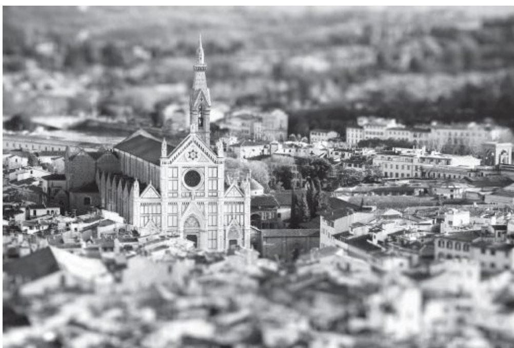
Fig. 4-24. With a tilt-focus lens, the in-focus part of the image can be manipulated to create interesting effects. The lens sometimes makes real-world scenes look like miniatures. This effect can also be simulated in post for footage shot normally.
