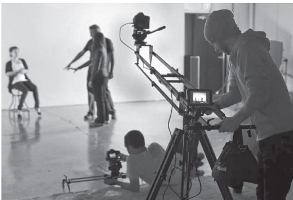
Fig. 9-9. The DSLR on the slider on the floor can make lateral movements; the camera on the jib arm can get high-angle shots and vertical movements (boom up or down). The operator watches a monitor mounted on the jib. (Amanda Kwok/SmallHD)
