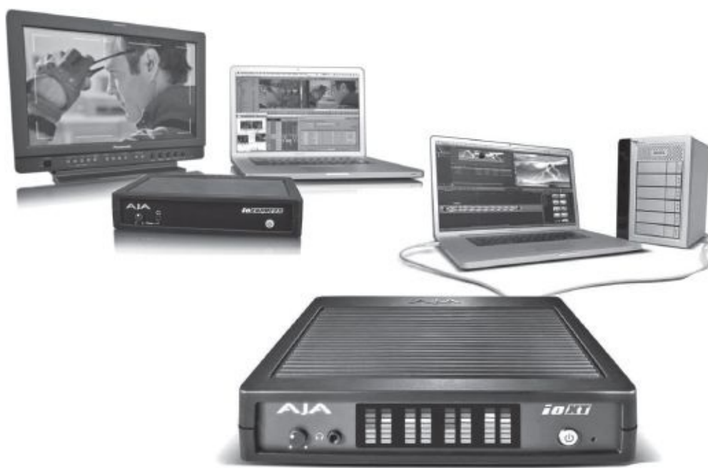
Fig. 14-4. (left) AJA Io Express supporting a broadcast video monitor. (right) AJA Io XT with Thunderbolt connectivity between a laptop and a RAID. Both products offer a wide range of input/output and monitoring options, as well as conversions between SD and HD formats. Can capture to ProRes, DNxHD, and CineForm codecs. (AJA Video Systems)
