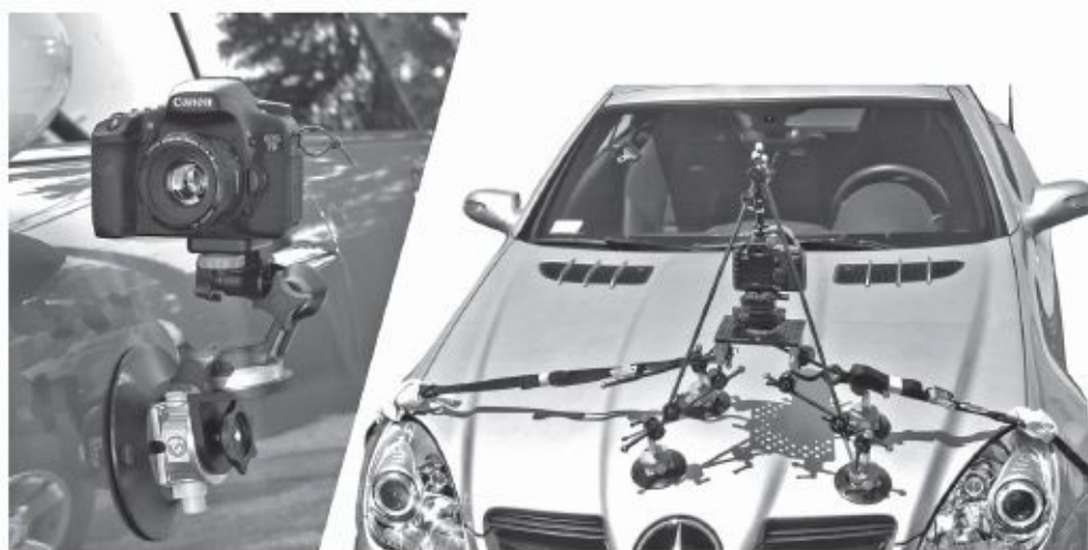
Fig. 9-47. Suction mounts can be attached to cars, windows, and nonporous surfaces. Car mounts should be set up by experienced persons using safety lines when possible. (Filmtools)
