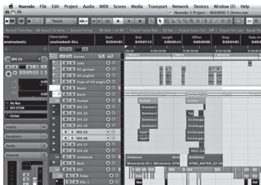
Fig. 15-3. DAWs, like the Nuendo system shown here, display audio clips on a timeline, much like NLEs do. (Steinberg Media Technologies GmbH)
