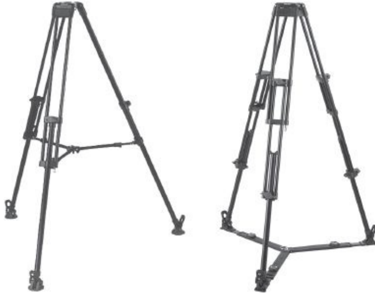
Fig. 9-39. (left) Tripod legs with the spreader mounted midleg can have an advantage when shooting on uneven surfaces. (right) Dual-stage legs (note three sections on each leg) can often go both lower and higher than comparable single-stage legs. This spreader is at ground level and attaches to the tripod feet. (Miller Camera Support)
