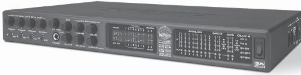
Fig. 10-12. The MOTU Traveler provides four mic inputs and a total of twenty channels of analog and digital inputs and outputs. A full-featured interface for recording to a laptop in the field. (MOTU, Inc.)
