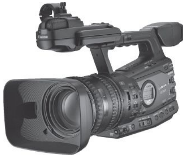
Fig. 1-18. Canon XF305 camcorder records MPEG-2 to CompactFlash cards. Three \frac{1}{3} -inch chips with 4:2:2 color. (Canon U.S.A., Inc.)
