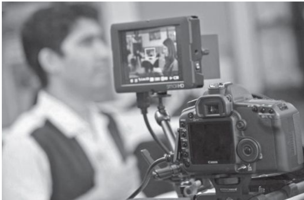
Fig. 2-22. Most DSLRs create small, highly compressed video files that are easy to store, but are sometimes easier to work with when converted to a less compressed format prior to editing. (Ally Shore/SmallHD)
