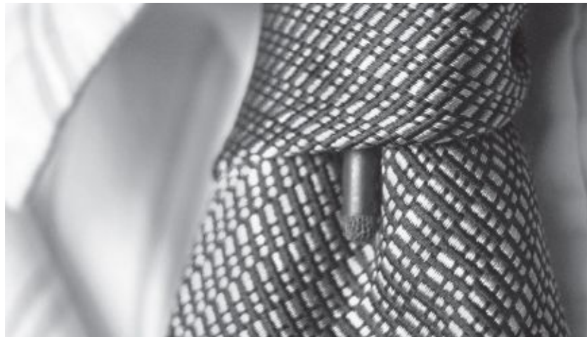
Fig. 10-26. The Sanken COS-11D lavalier has a very small capsule that can be hidden in clothing or hair. The mic would normally be tucked under the tie's knot to hide it. Also comes with a rubber sleeve that can be taped inside clothing. (Steven Ascher)
