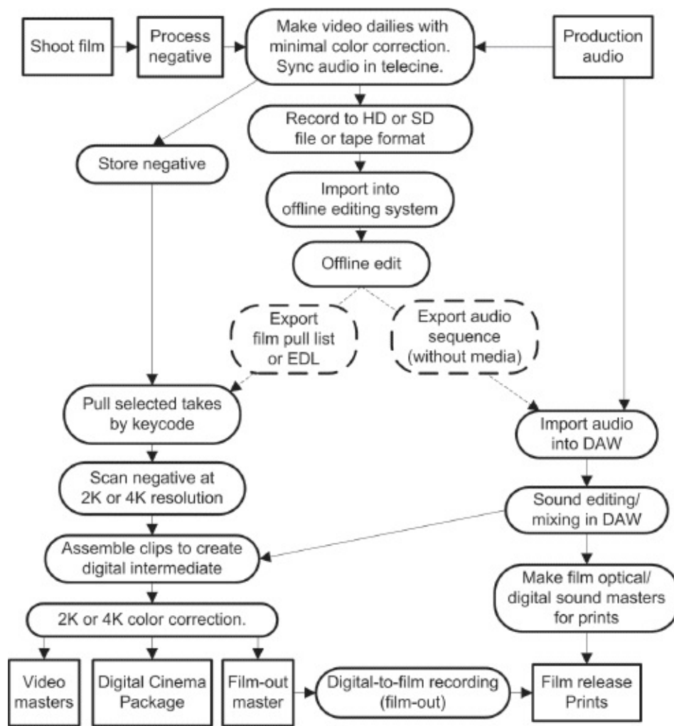
Fig. 16-4. Scenario Two. A possible route for shooting film, transferring to video dailies for the offline edit, then scanning the film to create a digital intermediate.
