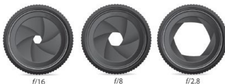
Fig. 4-8. Iris diaphragm. As the blades of the iris open, more light passes through the lens.
