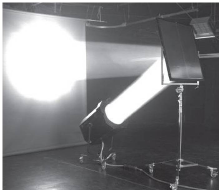
Fig. 12-21. A light source can be softened by bouncing it and/or by projecting it through diffusion
