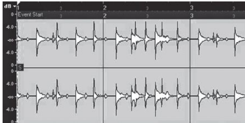
Fig. 14-24. Audio waveforms. A visual representation of a clip's sound, waveforms make some editing tasks easier. Shown here, stereo tracks of a percussive drum sound. The height of each waveform above the centerline corresponds to loudness. (Steinberg Media Technologies GmbH)
