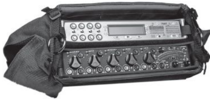
Fig. 10-30. Sound Devices 788T twelve-track, high-end audio recorder, shown with 552 mixer. The 552 mixer can also record digital audio internally to SD or SDHC media. (Sound Devices, LLC)
