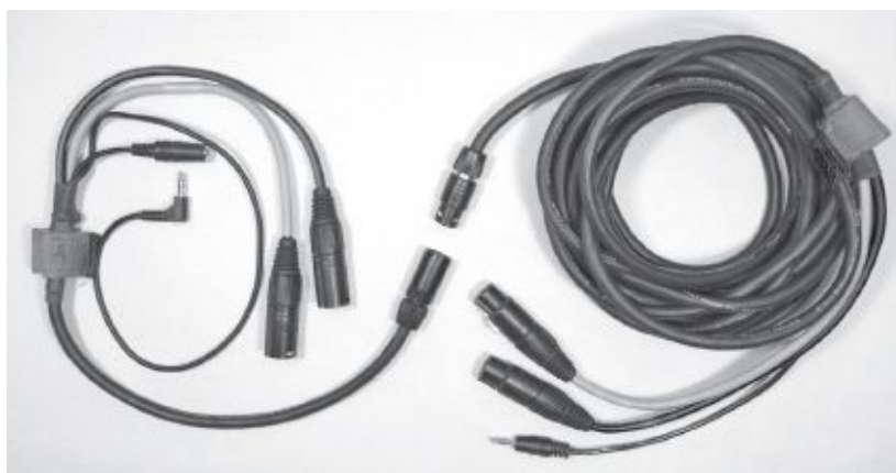
Fig. 11-3. Breakaway cable. The part of the cable on the right plugs into the mic mixer's output. The part on the left is the pigtail that plugs into the camera's input. In the middle is a breakaway link for quickly disconnecting the camera from the mixer when needed. Also included is a headphone feed from the camera to the mixer.
