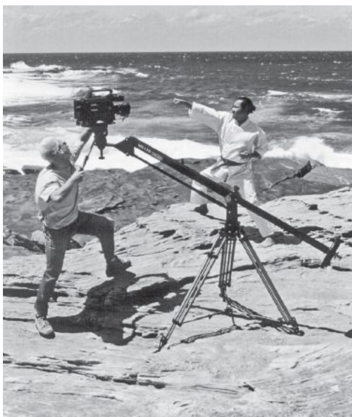
Fig. 9-43. Compact jib arms can be used for location and studio work, and can be mounted on a tripod or a dolly. (Miller Camera Support)
