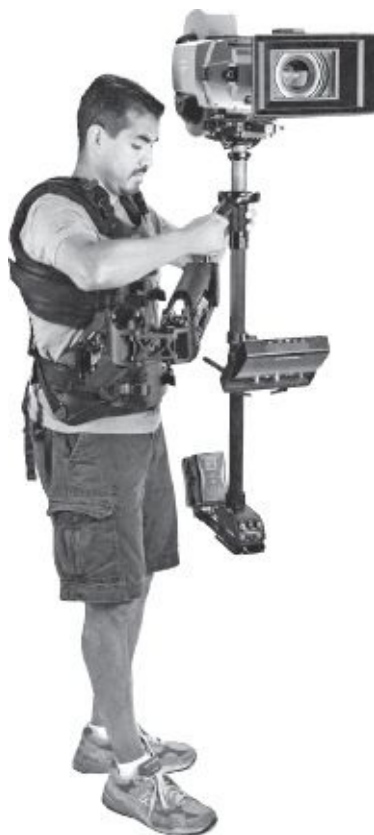
Fig. 9-48. Steadicam. The camera floats smoothly, isolated from shocks or jarring with springs in the support arm. The operator wears a harness and watches a small monitor mounted on the Steadicam. Steadicam and Glidecam also make smaller, handheld systems for small cameras (see Fig. 1-15 ). (The Tiffen Company)
