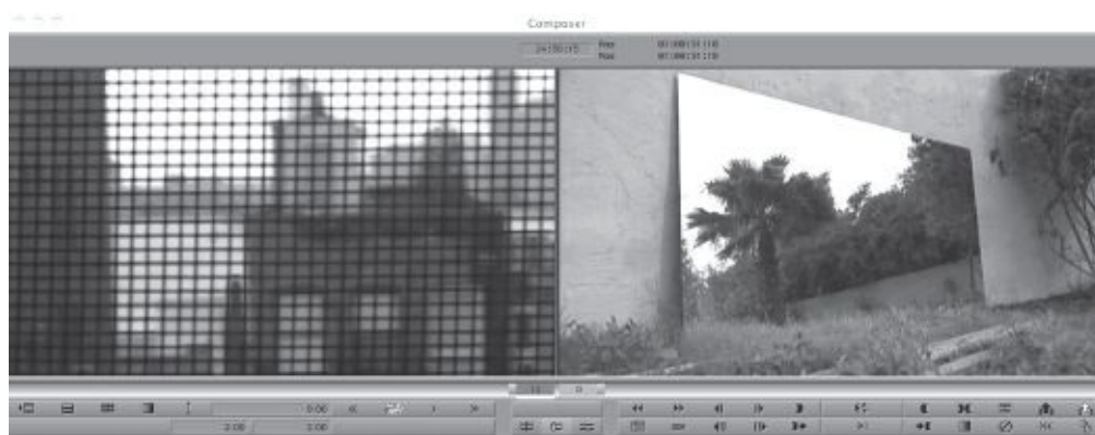
Fig. 14-21. Trim mode. This Avid trim tool displays the last frame of the outgoing clip and the first frame of the incoming clip. You can select to trim the ends of either or both clips. (Avid Technology, Inc./Steven Ascher)
