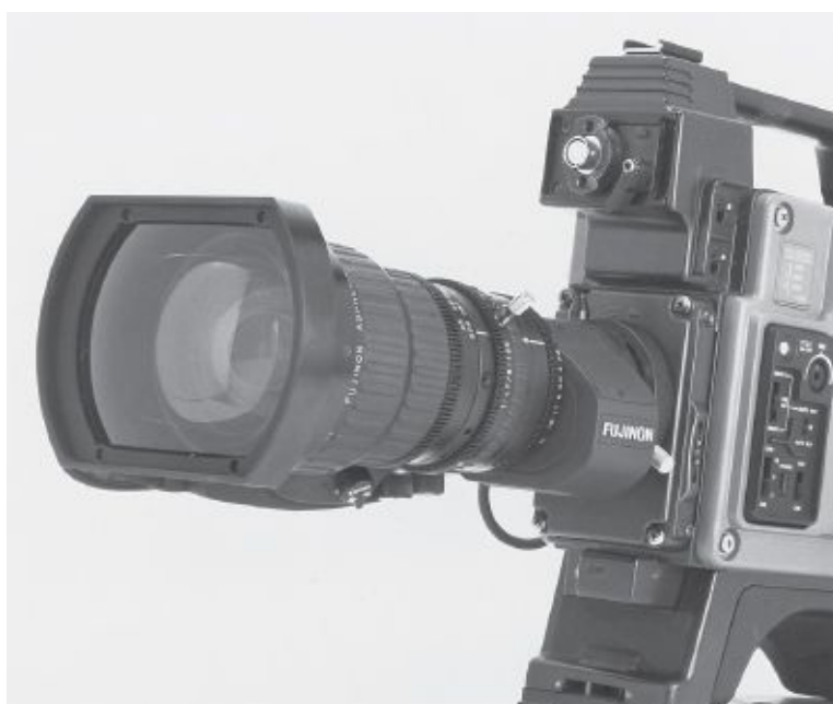
Fig. 4-19. Century Double Aspheric 0.6x wide-angle adapter mounts on the front of the lens. With this adapter you can't zoom during shots, but other Century adapters do permit full zooming. (Fletcher Chicago/Schneider Optics)
