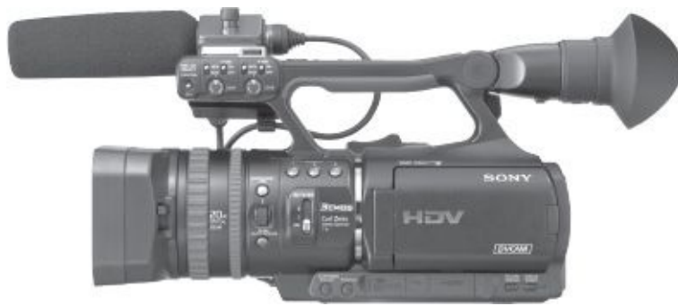
Fig. 1-20. Sony HVR-V1U. Records HDV as well as DVCAM and DV to tape cassettes and an optional external hard drive. Three 1/4-inch CMOS sensors. (Sony Electronics, Inc.)
