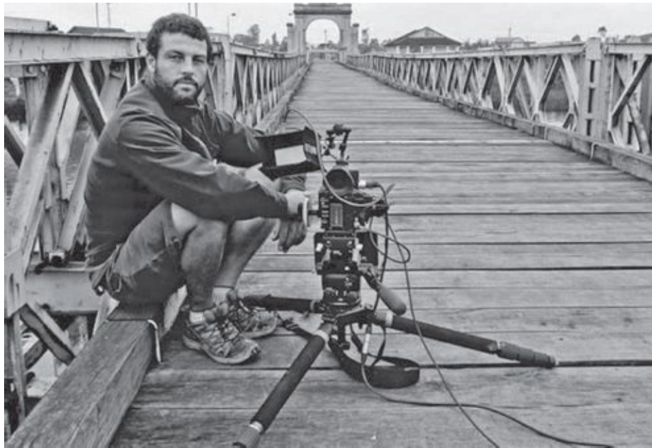
Fig. 9-40. A tripod that allows the legs to be spread wide permits low-angle shots. An external monitor makes viewing easier when the camera is low or high. (Toby Ralph/SmallHD)
