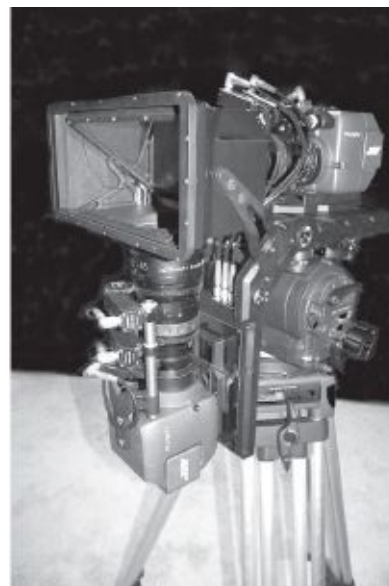
Fig. 9-54. Mirror 3D rig in which the two cameras (ARRI Alexas) shoot through a partially reflecting mirror. (Photo by David Leitner)
