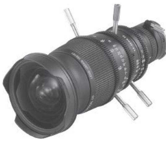
Fig. 4-17. Cine-style zooms (also called cinema- or film-style zooms) typically offer manual zoom, focus, and iris control, and have large geared teeth to accept an external zoom motor and/or a follow-focus device if desired. (Fujinon, Inc.)
