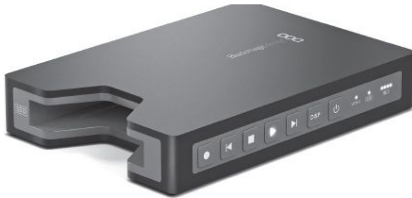
Fig. 5-30. Blackmagic Design's HyperDeck Shuttle is a compact video recorder that can capture uncompressed 10-bit HD or SD files to removable flash media SSDs. Connects to a camera via HDMI, HD-SDI, or SDI. Uncompressed files in a QuickTime wrapper are compatible with most editing systems, and material can be edited directly from the SSD. (Blackmagic Design)
