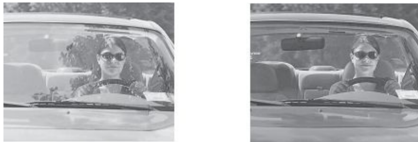
Fig. 8-8. (left) Without polarizer. (right) With polarizer filter. The polarizer minimizes the reflections from the windshield. (Schneider Optics)
