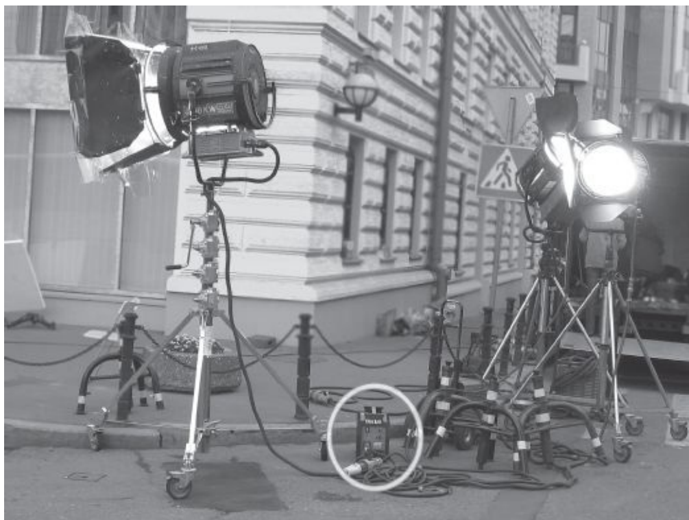
Fig. 12-11. HMI lights being used outdoors. Note the ballast unit (circled). HMIs are an efficient
