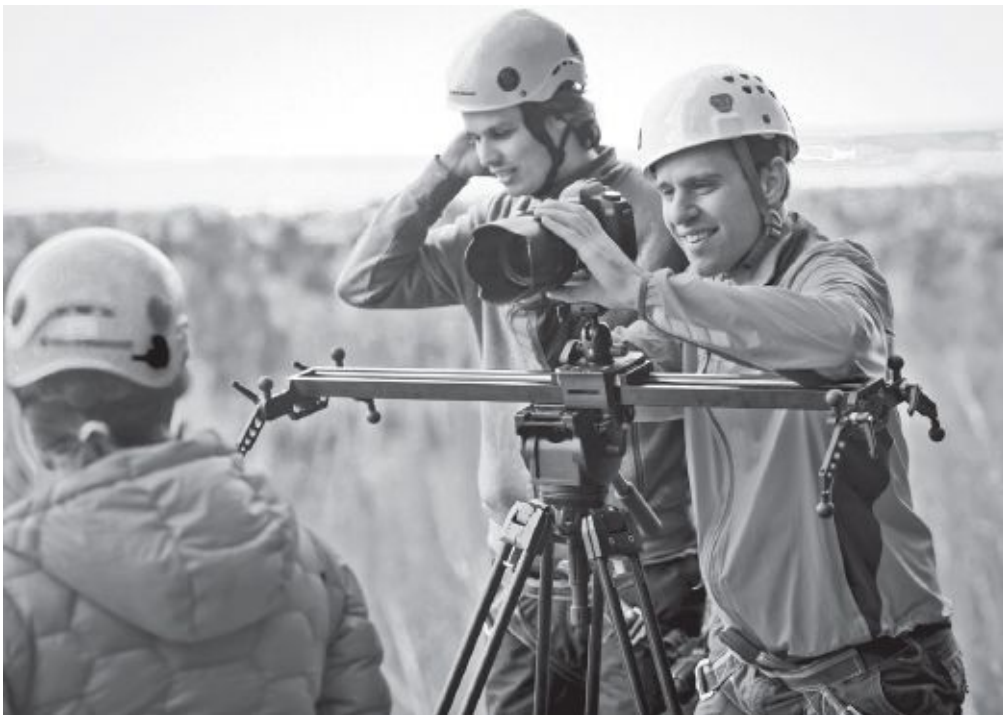
Fig. 9-46. Cinevate slider permits lateral or vertical moves. Can be mounted on a tripod or on the ground. When doing any kind of camera move, placing the subject or objects in the near foreground helps accentuate the sense of movement. See also Fig. 1-19 . (Cinevate)
