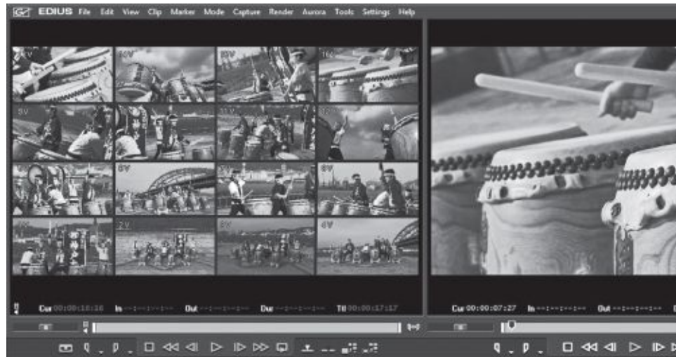
Fig. 14-29. Multicam editing. For shoots in which multiple cameras cover the same action (like a concert shoot), some NLEs allow you to load the different camera angles in the same timeline and easily switch between them to create the edited sequence. Shown here, Edius NLE (with lines added for clarity). (Grass Valley)
