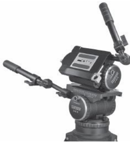
Fig. 9-6. The Cartoni Dutch head enables you to mount a second fluid head perpendicular to the first, allowing side-to-side as well as front-to-back tilts. (Cartoni)
