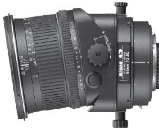
Fig. 4-23. Tilt-focus or perspective control (PC) lens. Tilt-shift lenses are sometimes used when shooting architecture to adjust perspective lines that appear to recede too fast. By tilting the lens axis, you can position the plane of focus at an angle to the camera instead of perpendicular to it. Tilting, shifting, and/or rotating the plane of focus allow you to bring an angled subject into even focus or create an out-of-focus effect (see Fig. 4-21 ). (Nikon, Inc.)
