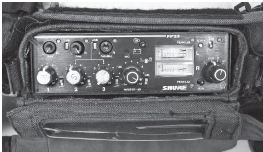
Fig. 10-29. Portable microphone mixer. The Shure FP33 is an affordable analog mixer, used by many crews over the years.
