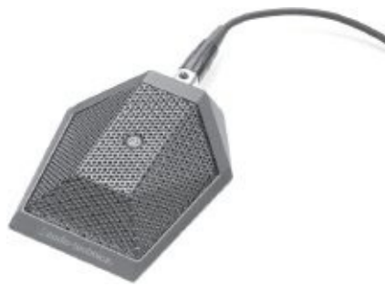
Fig. 10-19. Mounted on a flat surface, a boundary mic uses the surface to boost its audio response. (Audio-Technica U.S., Inc.)
