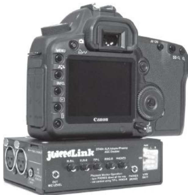
Fig. 10-14. The juicedLink DT454 preamp offers many enhancements for recording audio with a DSLR. Has four mic inputs (XLR and 3.5 miniphone stereo), phantom powering for mics, audio meters, and headphone jack. Provides manual gain control and can disable the camera's AGC. (juicedLink)
