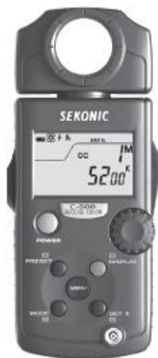
Fig. 8-5. Color temperature meter. Sekonic C-500 is a three-color meter that can be used with digital cameras and film. Can display color temperature in degrees kelvin or as a color-compensating (CC) index for selecting appropriate filters. (Sekonic)
