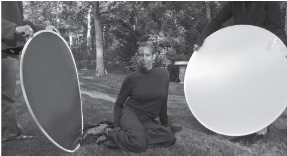
Fig. 12-22. Flexfill reflectors. Useful for filling shadows and reducing lighting contrast. Available in different surfaces: white maintains the character of the light; silver for more punch over longer distances; gold for adding warmth (shadows lit by skylight can sometimes look blue); translucent softens the light (when placed between light source and subject). Flexfills collapse to roughly one-third size when not in use. (Allen Green)
