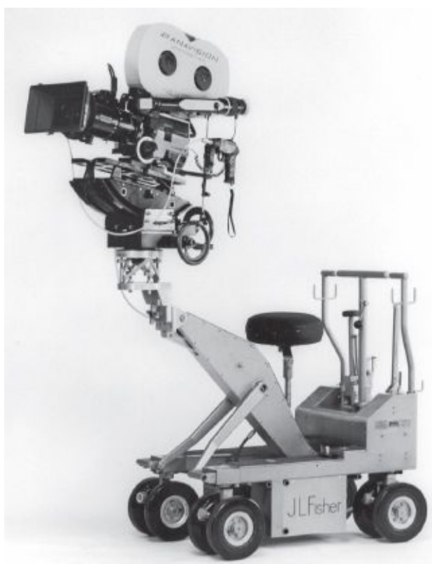
Fig. 9-42. Dolly with boom permits vertical as well as horizontal movements. (J. L. Fisher, Inc.)
