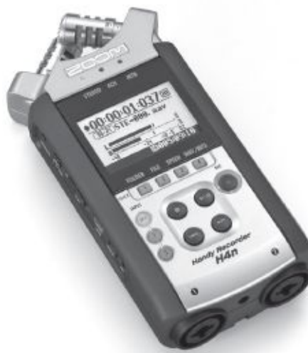
Fig. 10-6. The Zoom H4n Handy Recorder is a small, affordable device that records up to four tracks to SD and SDHC cards using built-in stereo mics or external mics input via either XLR or phone connectors.
