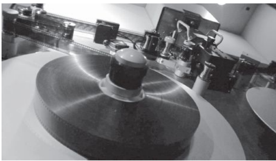
Fig. 16-6. The Spirit DataCine series of high-resolution scanners can output HD and SD video formats, and some can output 2K and 4K DPX data files. (DuArt Film and Video)
