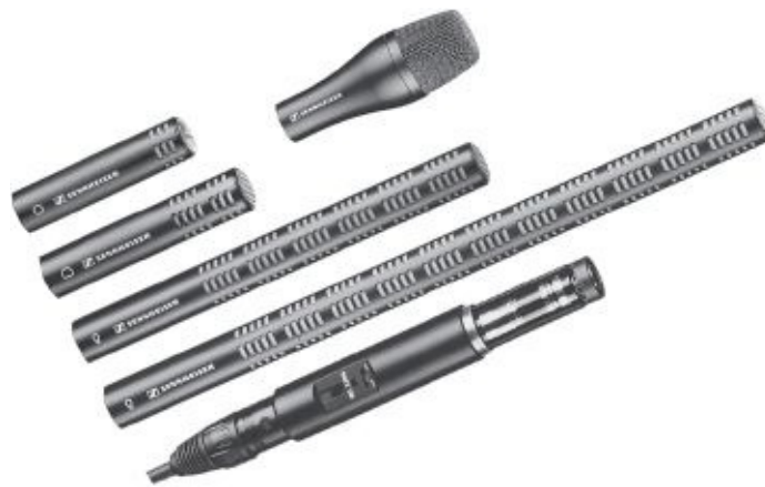
Fig. 10-18. Sennheiser K6 modular condenser microphone system. The powering module is at bottom (works with internal batteries or phantom power). Interchangeable mic heads range in directionality from supercardioid to omni. (Sennheiser Electronic Corp.)
