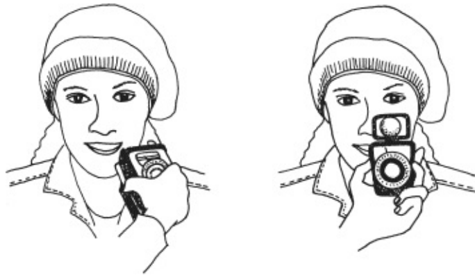
Fig. 7-11. (left) The reflected meter is pointed at the subject from the direction of the camera. (right) The incident meter is held in the same light as the subject and pointed toward the camera. (Carol Keller)
