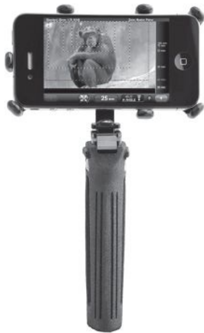
Fig. 9-28. A director's viewfinder allows you to view a scene with different focal length lenses, to get a feel for what focal length you want to use on the camera. This iPhone version combines a Zacuto handgrip with the Artemis director's viewfinder app. Director's finders are helpful for scouting locations and planning shots. (Zacuto USA/Chemical Wedding)
