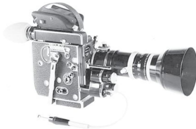
Fig. 6-5. Bolex H16 Reflex 16mm camera. Beam-splitter reflex with nondivergent lens turret. Spring-wound motor capable of single-frame operation. This camera accepts 100-foot internal loads or an external magazine. It has a 135-degree variable shutter. (Bolex)
