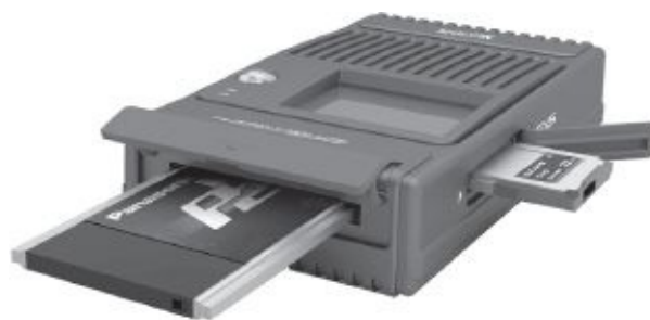
Fig. 3-7. This Nexto DI portable backup device can transfer the contents of a P2, SxS, or CompactFlash card to two hard drives simultaneously, with error checking. Allows previewing files and downloading in the field without a computer. (Nexto DI Co., Ltd.)
