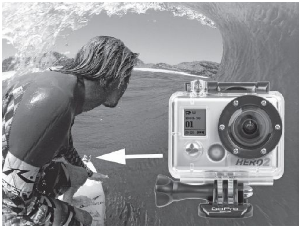
Fig. 2-8. The GoPro Hero2 is a small, waterproof HD camera that can be mounted on a surfboard, helmet, or vehicle for action scenes. (GoPro)
