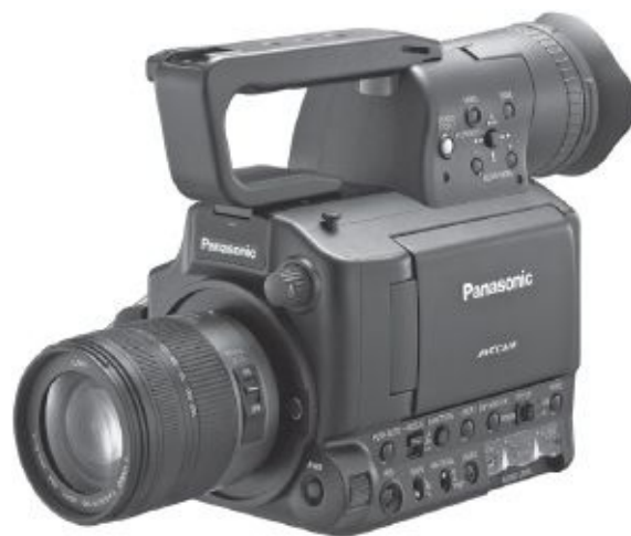
Fig. 3-6. Panasonic AG-AF100. Four Thirds CMOS sensor. Records AVCCAM internally to SDXC cards. Can output uncompressed 4:2:2 via HDMI for external recording. (Panasonic Broadcast)
