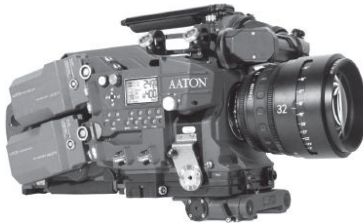
Fig. 2-20. The Aaton Penelope can shoot 35mm film, and replacing the film magazine with a "Digital-Mag" makes it a high-end digital cinematography camera. The Delta-Penelope can record uncompressed RAW as well as edit-ready, low-res proxy files. (AbelCine)
