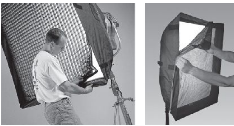
Fig. 12-26. (left) Cloth grid eggcrate being mounted on a large Chimera lightbank to reduce spill and direct light mostly toward the subject. (right) Using a scrim to reduce the output of a soft box. (Chimera)
