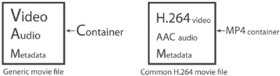
Fig. 5-32. A digital movie file is made up of video, audio, and metadata packaged inside a container
