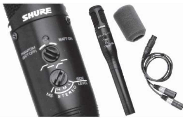
Fig. 11-16. Shure VP88 microphone. Versatile mic that can output an M-S signal or can be switched internally to provide a stereo (X-Y) output with a choice between low, medium, or high stereo effect. Comes with a splitter cable for outputting the two channels. Use both output connectors for M-S or stereo output, or use just one in the M-S mode to record a mono signal from the cardioid capsule or the figure-eight capsule. (Shure Brothers, Inc.)
