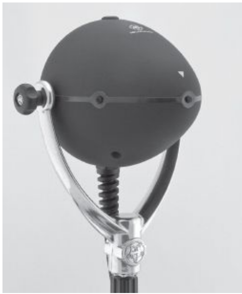
Fig. 11-18. Holophone's H2-Pro 5.1 can capture up to five channels (left, center, right, left surround, right surround, and low frequency) in one mic body. Outputs each channel via a separate XLR cable to a mixer or recorder. Other models can encode the 5.1 channels to two-channel stereo for recording in a typical camera. (Holophone)
