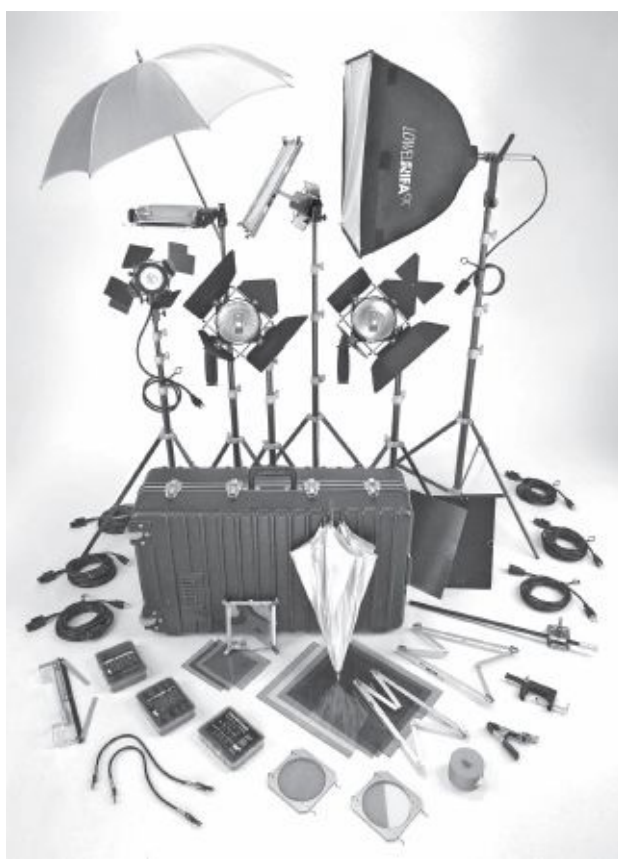
Fig. 12-28. Lowel Super Ambi Kit. Location package includes two Omni-lights (650-watt-maximum open-faced spots); two Tota-lights (1,000-watt-maximum broads) with umbrellas; one Rifa eX 55 soft box; one Pro-light spot. Accessories include stands, flags with flexible stems, scrims, door/wall brackets, clamps, gel frames, etc. Everything fits into the carrying case. (Lowel Light Mfg., Inc.)
