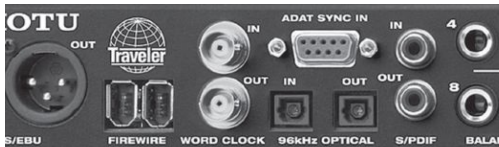
Fig. 10-13. The rear panel of the Traveler provides a good view of various connectors used for digital audio. From the left: XLR (used here for AES/EBU); FireWire; BNC (used here for word clock); nine-pin (used here for ADAT), TOSLINK (for S/P DIF optical); RCA (used here for S/P DIF coaxial); 1/4-inch phone jack for balanced analog input. (MOTU, Inc.)
