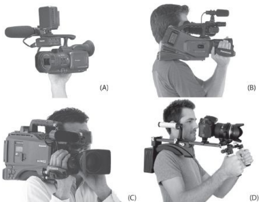
Fig. 2-16. (A) A small handheld camera is light and portable but can be hard to hold steady. (B) This camera perches on the shoulder, which increases steadiness, but a lot of the weight is on your right arm, which can get tiring. (C) A shoulder-mount camera that balances on the shoulder can be steadier and sometimes more comfortable for handheld work, even if it’s heavier. (D) Some shoulder braces for small cameras place batteries or counterweights behind the back to help balance the camera.
