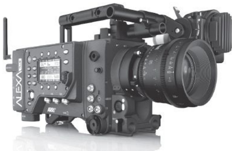
Fig. 1-23. ARRI Alexa digital cinema camera. Single Super 35 sensor. Accepts standard PL-mount 35mm cine lenses. Can record RAW data, RGB 4:4:4, and other formats including ProRes. One of the most popular cameras for feature film production. (ARRI, Inc.)
