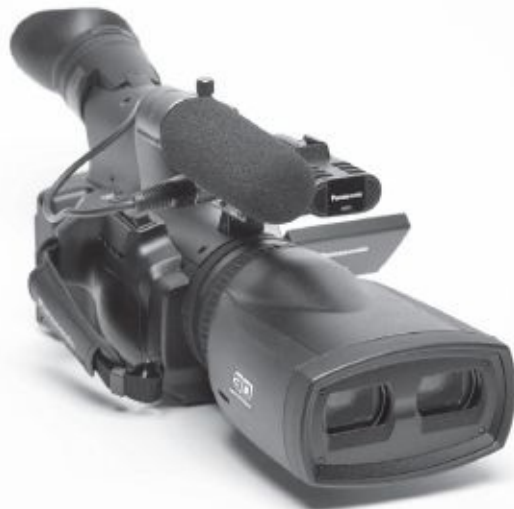
Fig. 9-51. 3D camcorder. The Panasonic AG-3DA1 has dual lenses and two 1920 x 1080 HD sensors. This kind of one-piece camcorder is easier to operate than 3D rigs that use two separate cameras. (Panasonic Broadcast)
