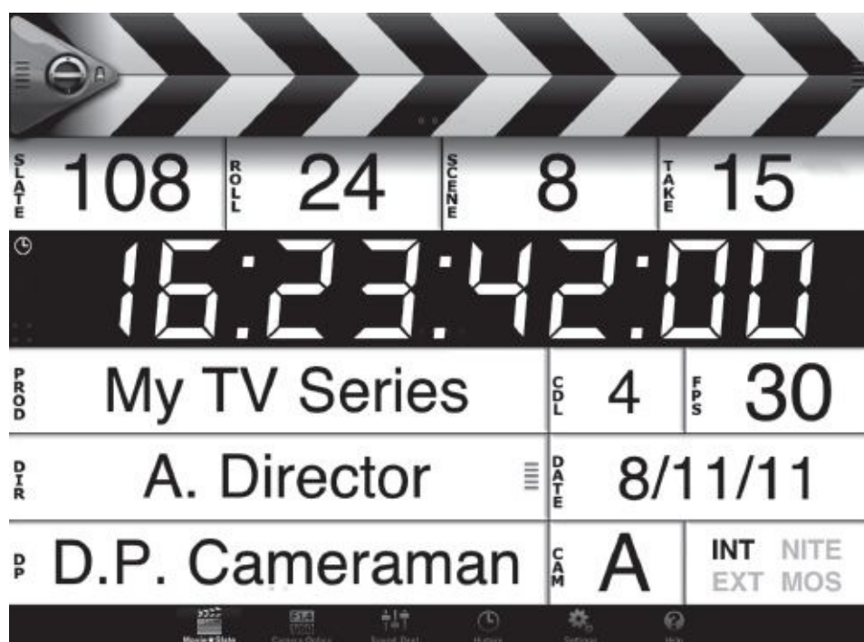
Fig. 9-30. MovieSlate app for iPhone or iPad. Displays time-of-day (TOD) timecode or you can jam timecode from an external source. A shot log—including scene and take info, notes, and other data such as GPS location—can be exported easily via the Web. A plug-in is available for generating detailed sound reports. (PureBlend Software)
