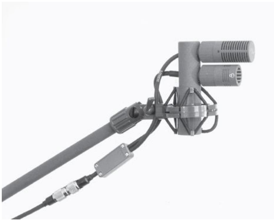
Fig. 11-17. Schoeps M-S setup showing separate cardioid and figure-eight mics that can be combined (matrixed) to create stereo. Schoeps makes very high-quality professional mics. (Posthorn Recordings, NY)
