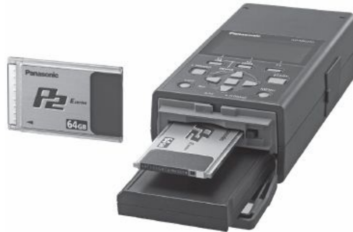
Fig. 2-17. (left) P2 card. These flash memory cards are about the size of a credit card and are available in various storage capacities. (right) The Panasonic AG-MSU10 unit can transfer the contents of a P2 card (in the upper slot) to a removable hard drive or SSD (in the tray below). Allows you to download cards in the field without a computer. (Panasonic Broadcast)
