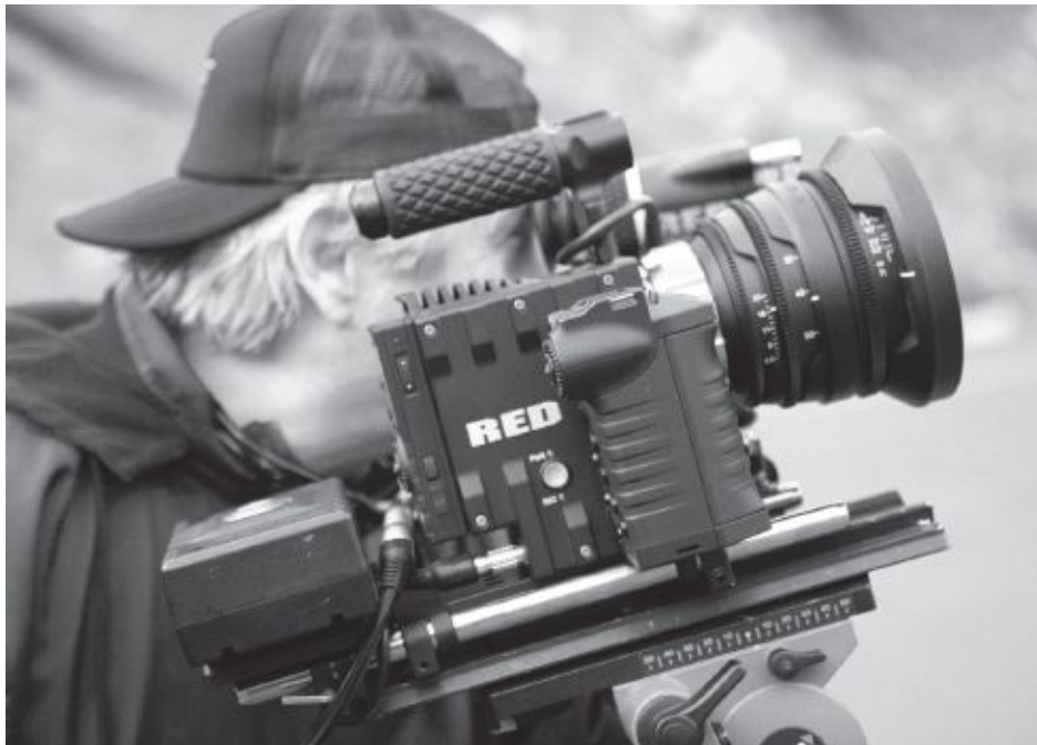
Fig. 1-24. RED's Epic DSMC (Digital Still and Motion Camera) has a 5K, Super 35 sensor. Acquisition formats include RAW and RGB 4:4:4. Can capture up to eighteen stops dynamic range with HDRx recording. Popular for features and adapts well to 3D. (RED)
