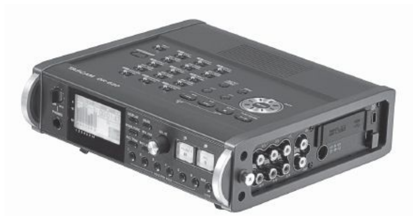
Fig. 10-5. Tascam DR-680 records up to eight tracks to SD cards. (TASCAM)
