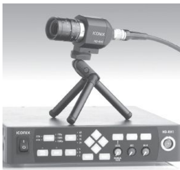
Fig. 3-5. Iconix camera and control unit. The camera head is a little bigger than a golf ball and can be used for hard-to-reach camera angles and point-of-view shots as well as stereoscopic 3D applications. Outputs 2K and most flavors of HD. (Iconix Video)
