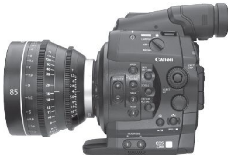
Fig. 3-13. Canon EOS C300 camera. Has a Super 35 sensor and records HD using the XF codec (MPEG-2, long GOP, 4:2:2 color) to CF cards. Supports HD-SDI output to external recorders or monitors. Available in Canon EF lens mount and PL-mount versions. (Canon U.S.A., Inc.)
