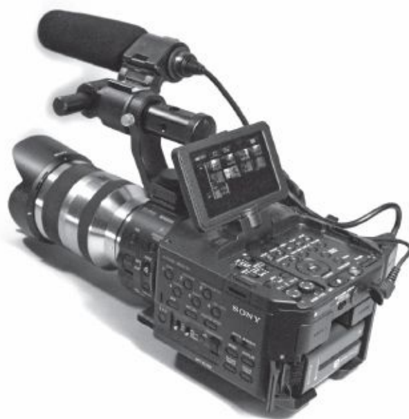
Fig. 1-17. Sony FS100 records AVCHD to memory cards and/or an SSD. Super 35 sensor (see Fig. 1-9 ).
