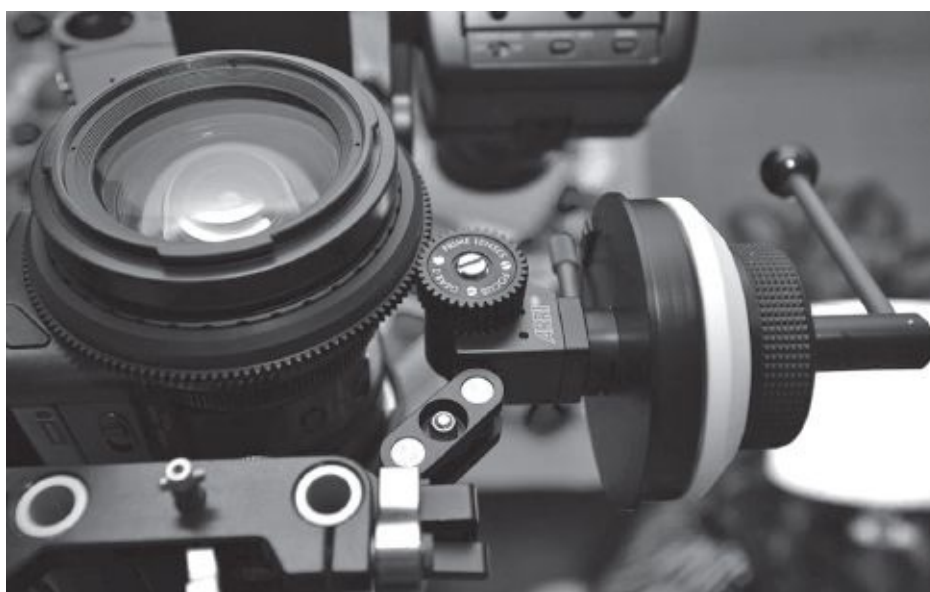
Fig. 4-15. The follow-focus device has a geared wheel that engages a toothed ring on the lens. If the lens has no gear ring, or the teeth are the wrong size, a ring can usually be added. Also see Fig. 1-3 . (Zacuto USA)
