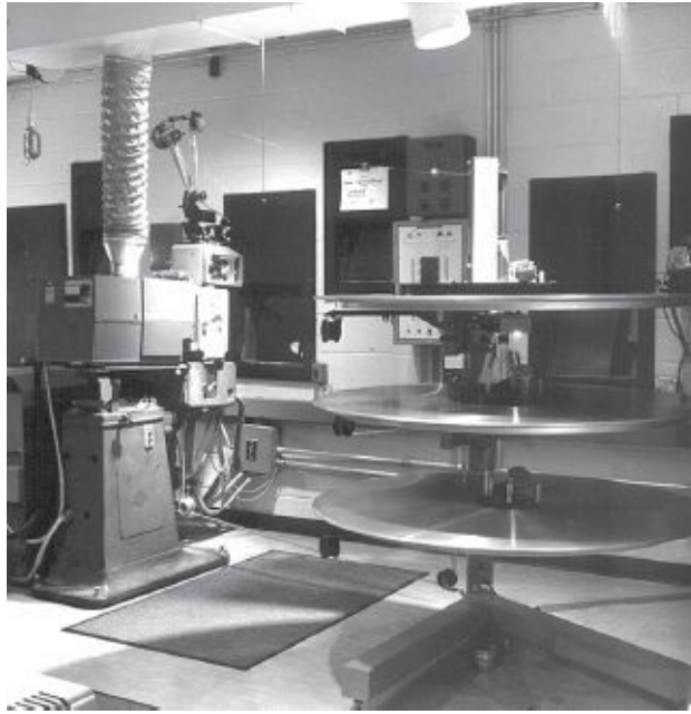
Fig. 16-17. Many theaters use a platter system so that an entire print can be spliced together, fed to the projector in one piece, and spooled up again. The projectionist only has to start the projector at the beginning and turn it off at the end. (Film-Tech.com)
