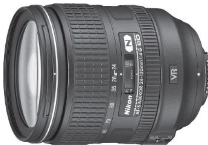
Fig. 4-18. Zooms designed for SLR or DSLR still cameras usually provide autofocus and auto-iris control through the camera (depending on the lens/camera combination). Manual overrides may be available, but the lens itself may have no manual iris control. Zooming is done manually. Some lens/camera combinations offer image stabilization. Often there are no distance markings on the lens for focus. (Nikon, Inc.)
