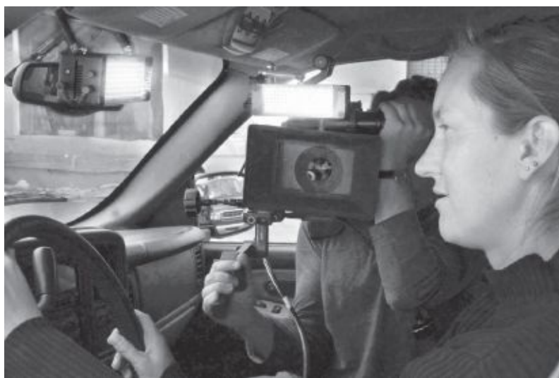
Fig. 12-15. Litepanels MiniPlus LED lights mounted on a car mirror and camera. LEDs are efficient lighting, available in daylight and/or tungsten balance, and fully dimmable with virtually no shift in color. LEDs are available in large and small panels. (Litepanels, Inc.)
