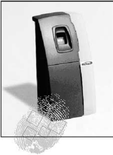
FIGURE 12.3 Plug-and-play fingerprint reader can confirm if people are who they claim to be, by matching fingerprint templates stored in a central database.
