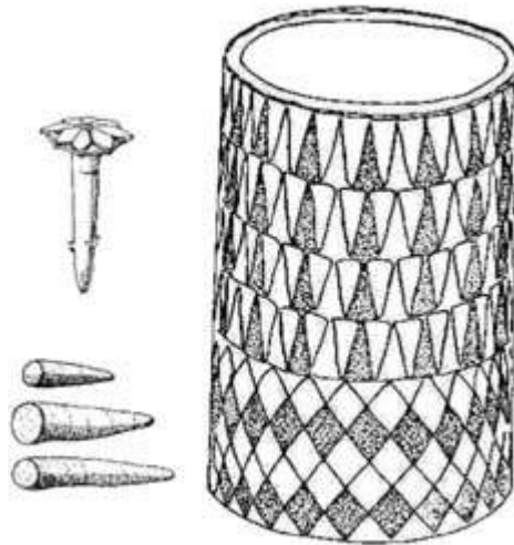
FIGURE 1.19 Brightly painted clay nails used by the Mesopotamian builders for decoration to hide the ubiquitous characteristics of the mud.
