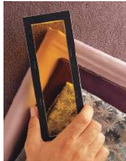
Figure 2.26 The yellow acetate lens allows the designer to see colors as older users might see them, as the eyes may become affected by a yellowing of the cornea. © Bradley H. Slade
