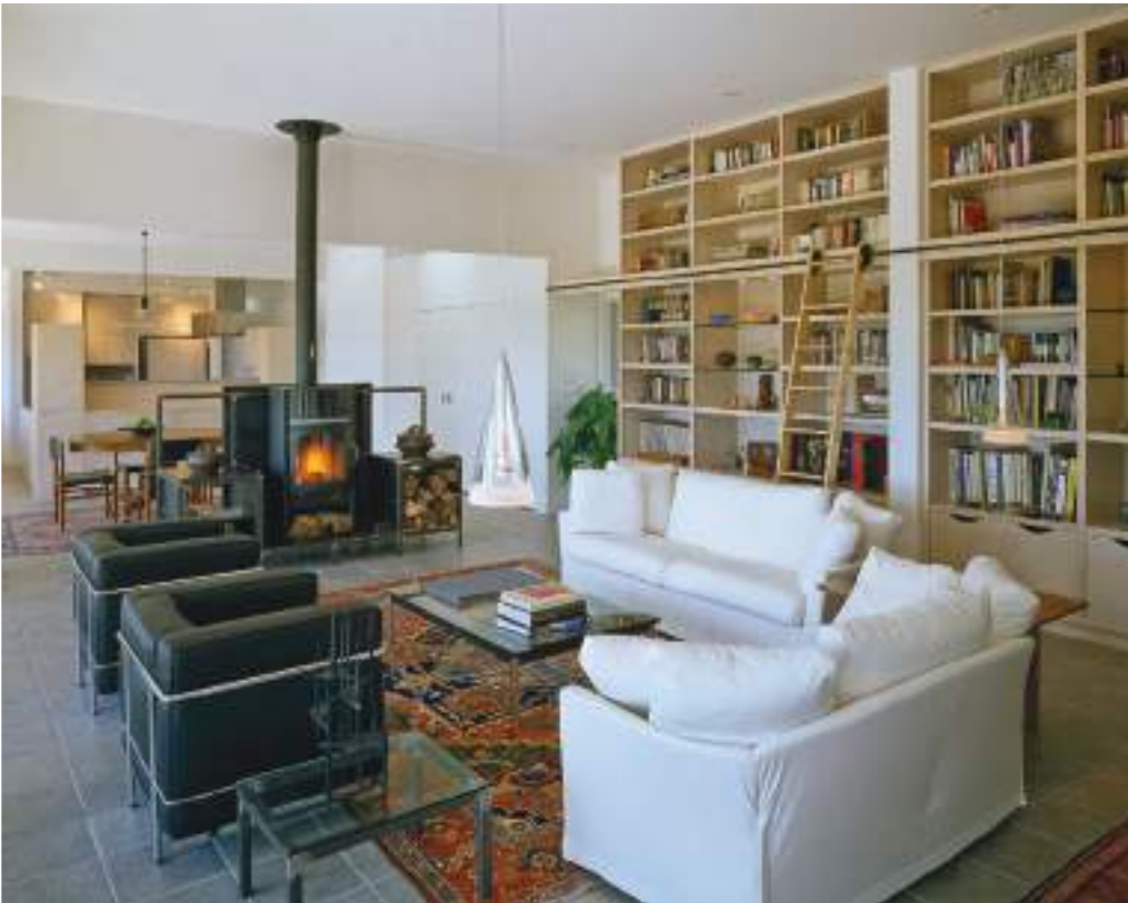
Figure 7.22 This contemporary wood-burning stove supplements heating and gives the owners a greater sense of self-sufficiency. Located in the center of this open plan space, the heat can radiate into both the living/conversation area and the kitchen and dining area. Design by Elliott Elliott Norelius Architecture/photo © Brian Vanden Brink
