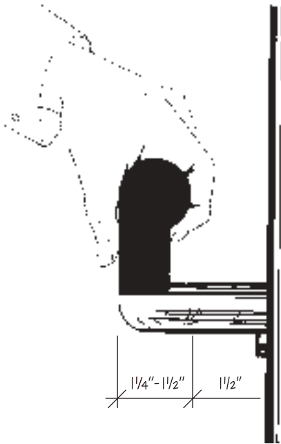
Figure 2.12 This handrail diagram shows the ideal size and shape for optimum universal design comfort. Handrails are essential for steadying and balancing for many individuals, including those who are ambulant disabled.
